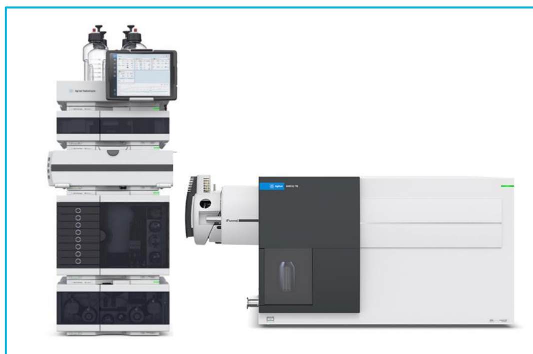
Figure 2: Infinity II Bio LC stack included a multisampler, column compartment with bio compatible switching valve, and high speed 1300 bar pump all made from bioinert material for improved detection limits for metal sensitive analytes. The 6495C LC/TQ was used in this method because the ion funnel improves detection limits.
